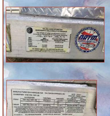
This trailer plate tells us that the Dalton Enterprises trailer is made in July 2011 and has a GVWR of 7000 pounds (3500 each of 2 axles). The VIN and Model are at the bottom.
