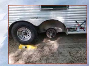
This trailer is up on a drive-up chock (which may be too short for some trailers - put a  $2 \times 6$  chock under it!) with tools ready as the tire is changed.
