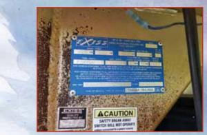
Reading the manufacturers plate, this is a GVWR (Gross Vehicle Weight Rating) of 9995 pounds. In the middle is information on the axles (2) and tires. The VIN number is on the bottom of the photograph along with the model.
